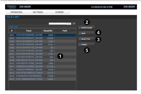
Press the **Mapping** button in the Hot Start screen or press the **Insert File** button in the Program screen to display the DN-900R file list and select files.
