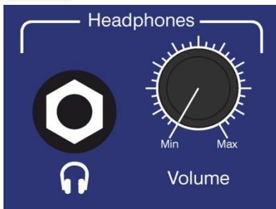
The headphone output is suitable to drive headphones with a minimum impedance of 16Ω
